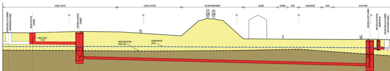
Schematic showing long section through siphon
