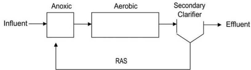
Figure 1.1 – Existing carbonaceous activated sludge process
