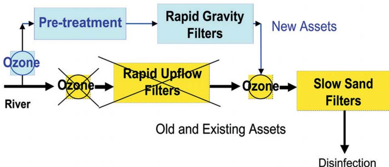
Schematic showing Fobney WTW Process Upgrade
