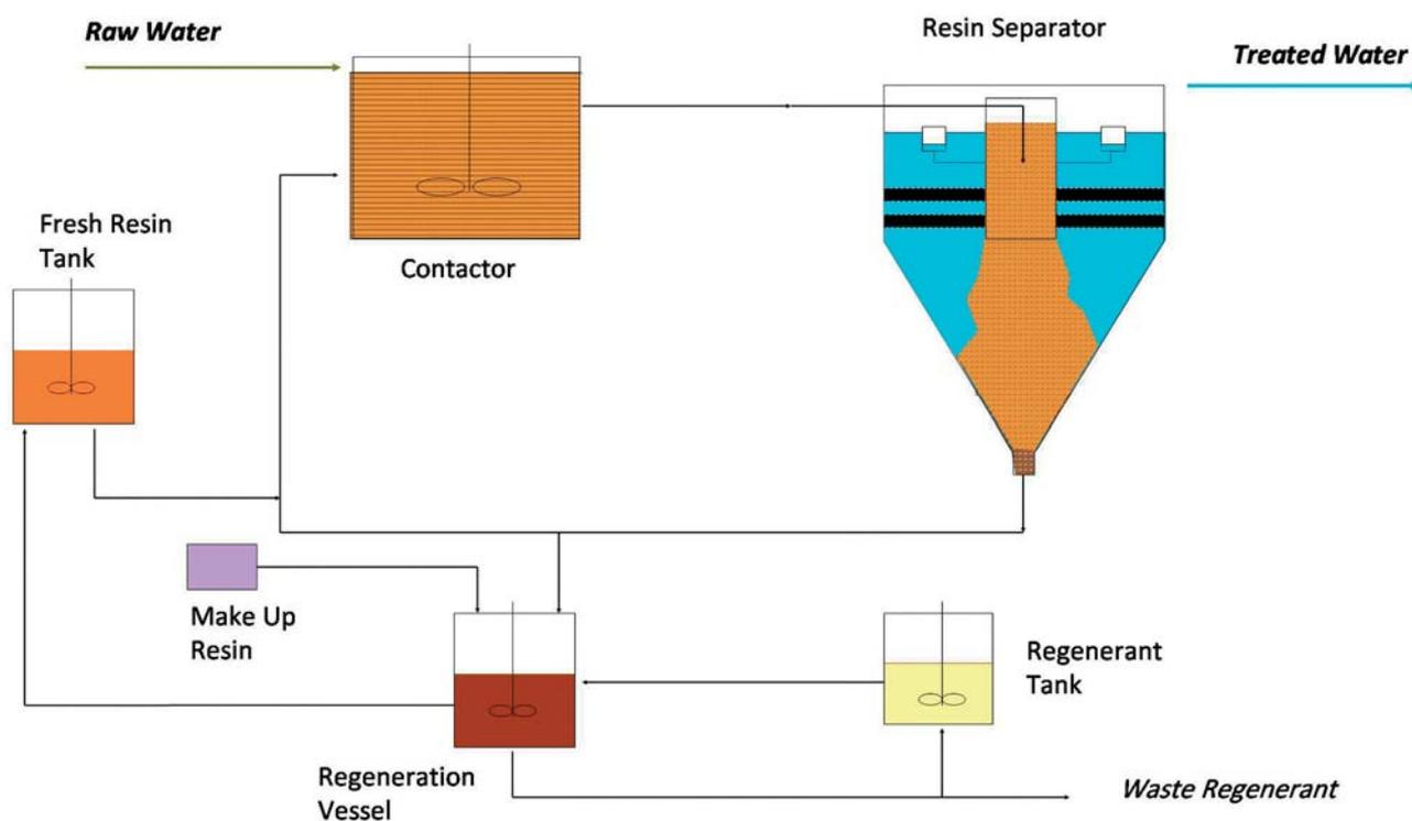
Process Flow diagram of the MIEX® Process
