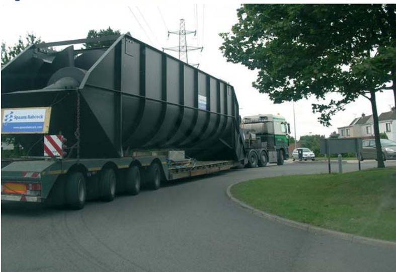
A packaged screw pump weighing 33 tons negotiates a roundabout in Llanelli on route for Cambrian Pumping Station. It is to provide storm water relief (1,600 litres per second) for Imtech on behalf of Welsh Water.
