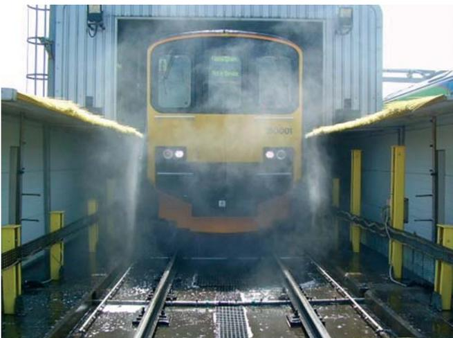
New underframe washer in operation (left) and cleaned train leaving Tyseley Depot (right)
