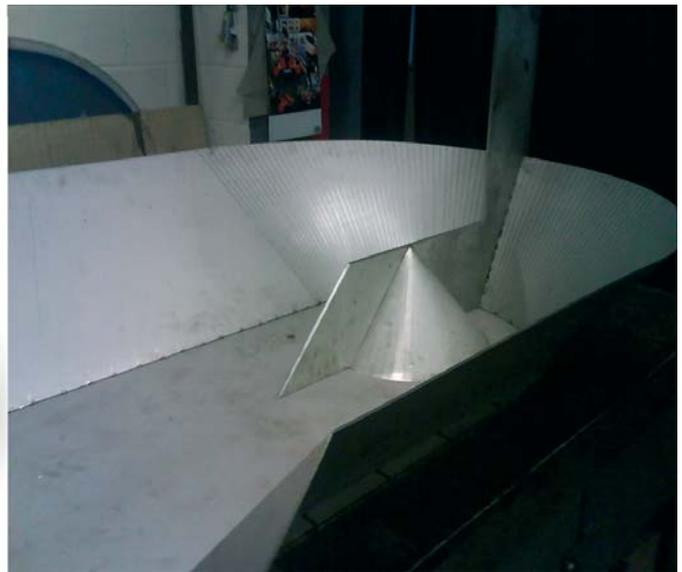
...and the completed stainless steel baffle Courtesy of South West Water
