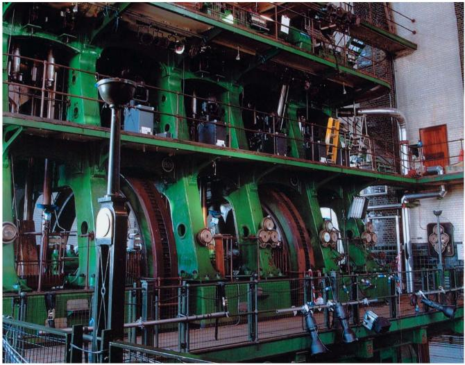
Engine number six - one of the two triple expansion engines at Kempton - nearing complete restoration (photo supplied by Great Engine Trust)
