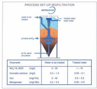
Process set-up Biofiltration (courtesy Paques)
