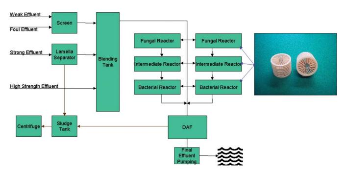
The Avlon works currently produces four effluent streams - Strong; Weak; High Strength & Foul
