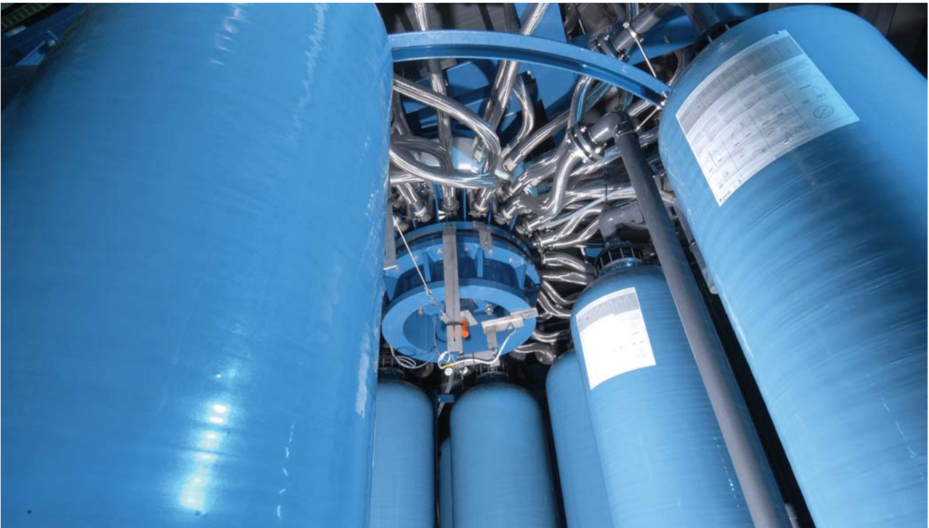
View of underside of ISEP valve at centre of turntable surrounded by resin vessels
