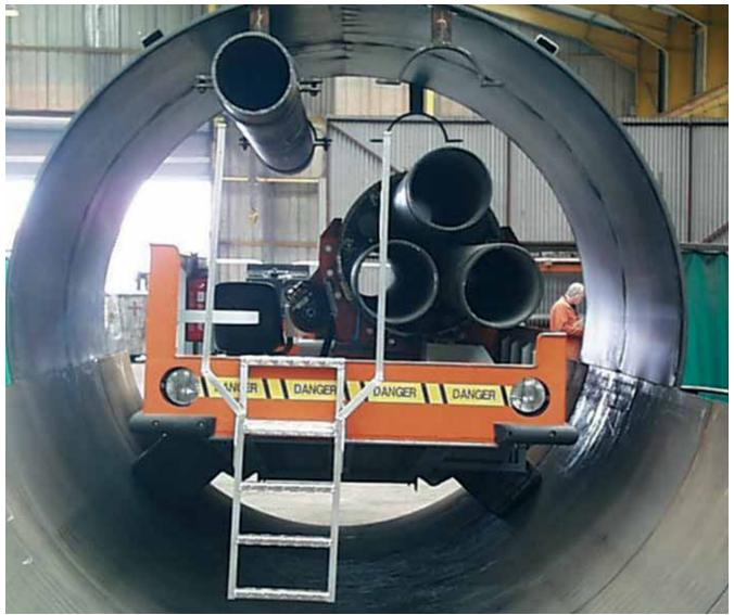
Unique tracked vehicles designed for removing old pipes and fitting new
