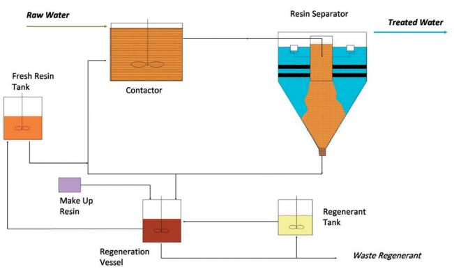
Process Flow diagram of the MIEX® Process
