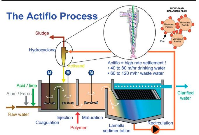
Picture above: General schematic of Actiflo® process.
