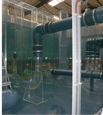
Perspex Model of Pumping Station
