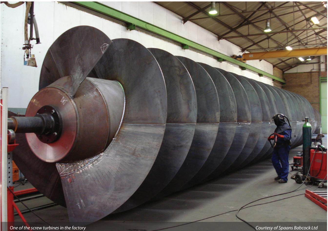
One of the screw turbines in the factory
