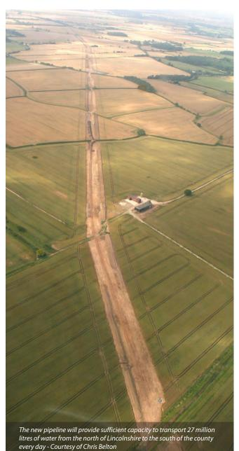
road locations, for the full length of the pipeline. Top soil stripping was done at a 28m width to mitigate the impact of the excavation on soil structure and ensure that the land can be returned back to its original state following installation of the pipeline. After preconstruction, land drainage was installed and welded pipe strings were laid out along the easement.
