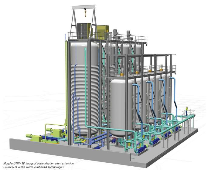
The original pasteurisation plant commissioned in 2007 comprised 8 (No.) reactor streams and ancillary equipment. The current contract for addition of 4 (No.) new reactor streams, was awarded to Black & Veatch in July 2010.
