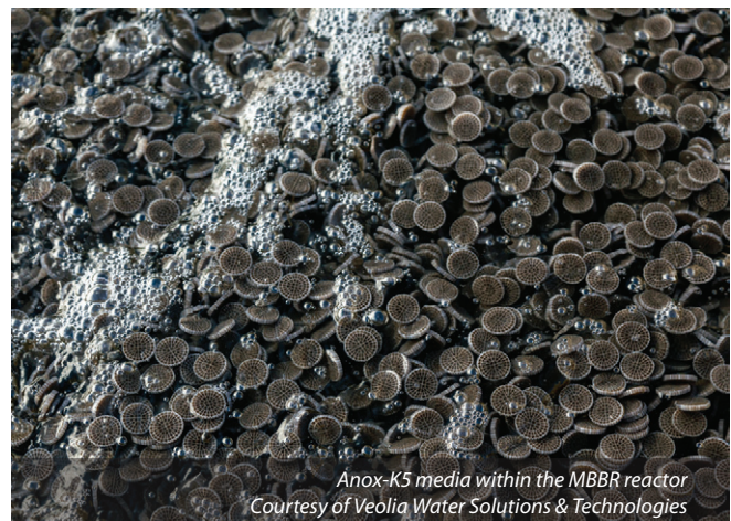
Moving Bed Biofilm Reactor - Courtesy of MGJV
