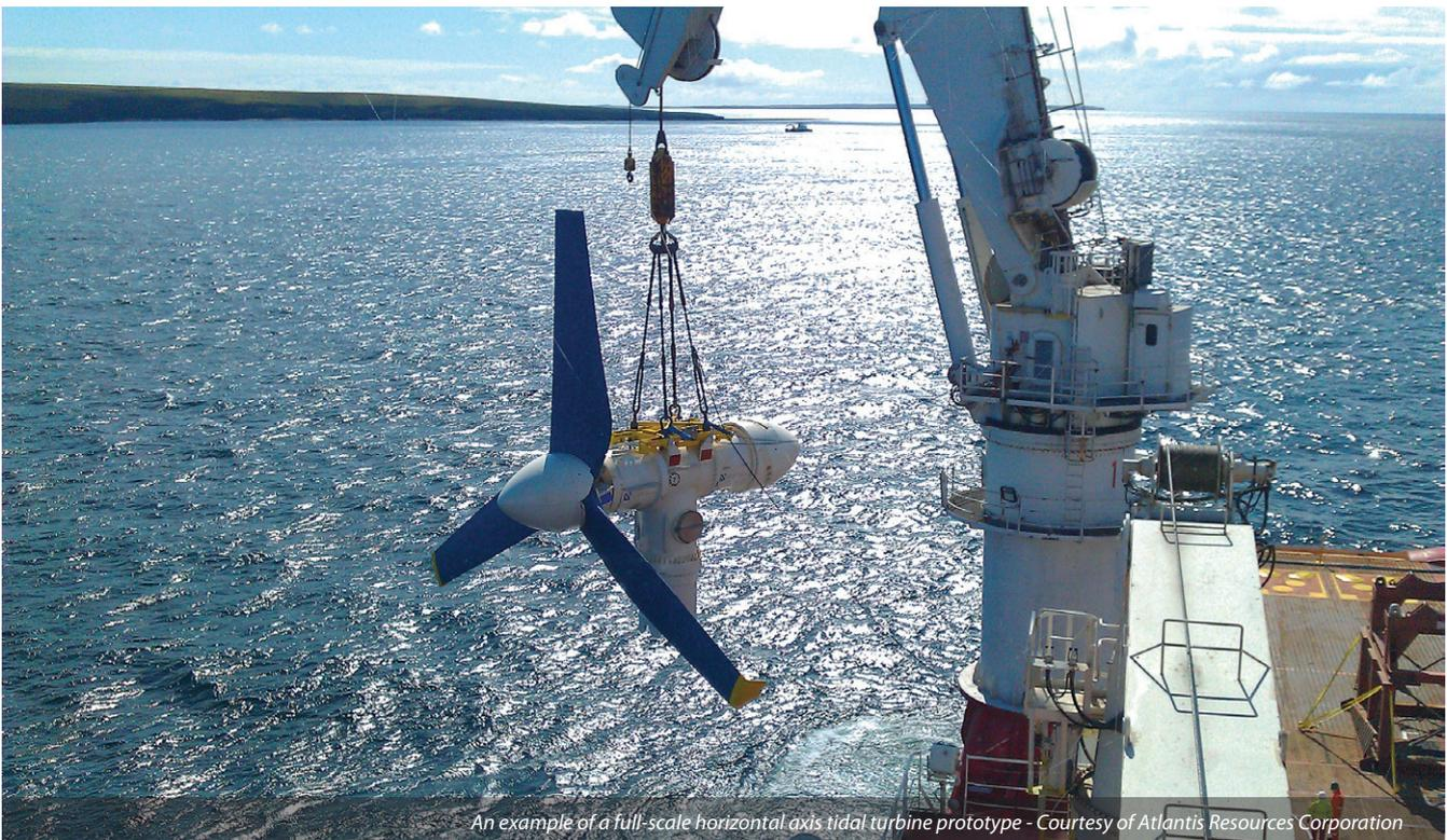
An example of a full-scale horizontal axis tidal turbine prototype - Courtesy of Atlantis Resources Corporation
