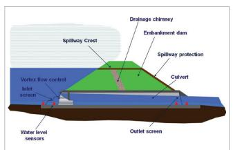
Typical cross section through dam and flow control structure Courtesy of CH2M HILL
