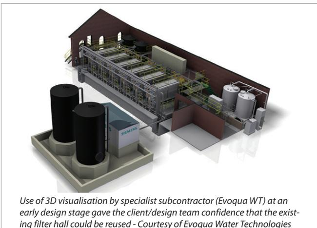
Use of 3D visualisation by specialist subcontractor (Evoqua WT) at an early design stage gave the client/design team confidence that the existing filter hall could be reused - Courtesy of Evoqua Water Technologies
