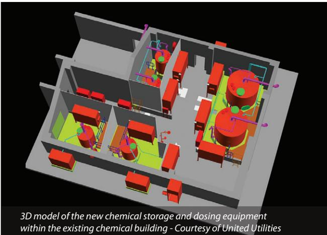
3D model of the new chemical storage and dosing equipment within the existing chemical building - Courtesy of United Utilities
