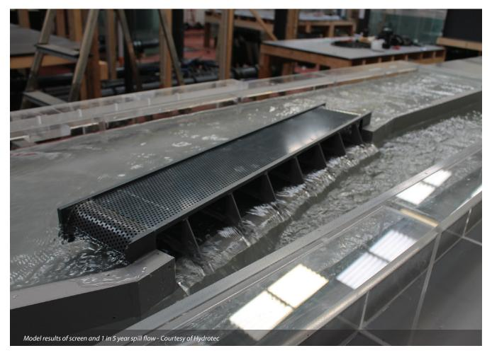
showing the layout of the existing culvert and proposed CSO. Hydrotec had previously investigated the operation of existing pump sumps, inlet works and other CSO screens.
