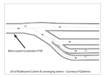
This dictated the location of the CSO chamber outside the Swindon STW boundary in an area owned by Swindon Borough Council with the overflow culvert passing under the B&Q car park.
