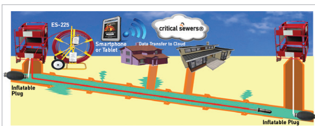
Figure 2. Electro Scan Testing and Current Trace - Courtesy of Electro Scan Inc
