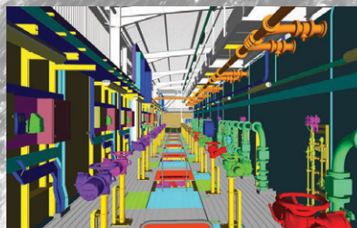
Removal of all valves and flow meters from lower level considered with suitable removable sections of floor to provide access - Courtesy of LOR
