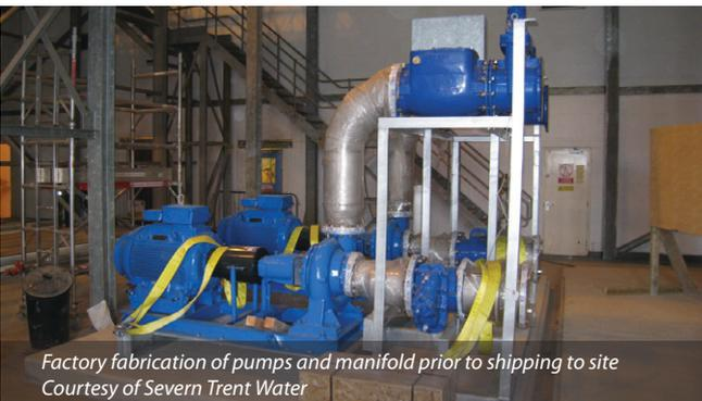
Factory fabrication of pumps and manifold prior to shipping to site
