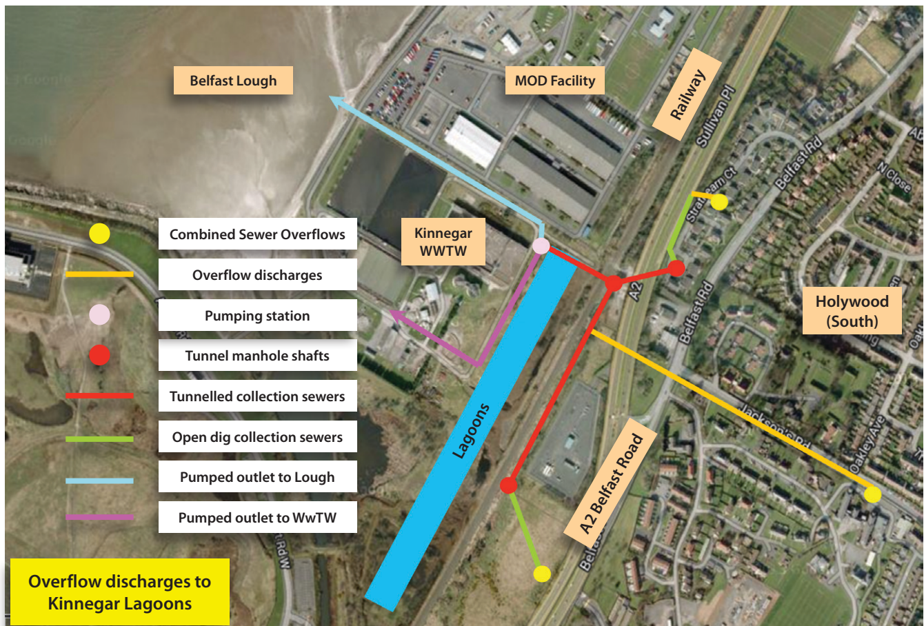
Location plan showing proposals for diversion of overflow discharges - Courtesy of NI Water
