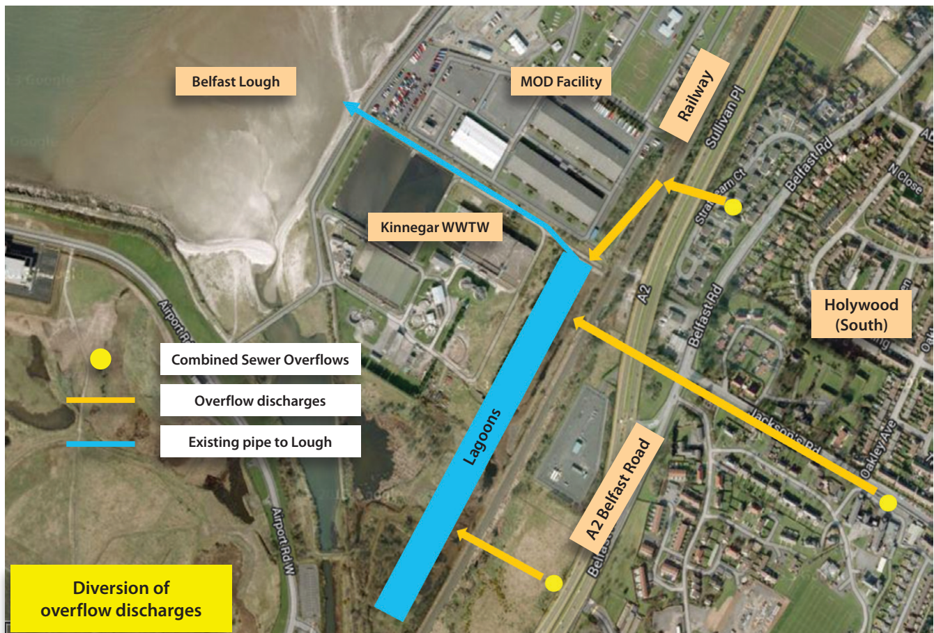
Location plan showing combined sewer overflow discharges to Kinnegar lagoons - Courtesy of NI Water
