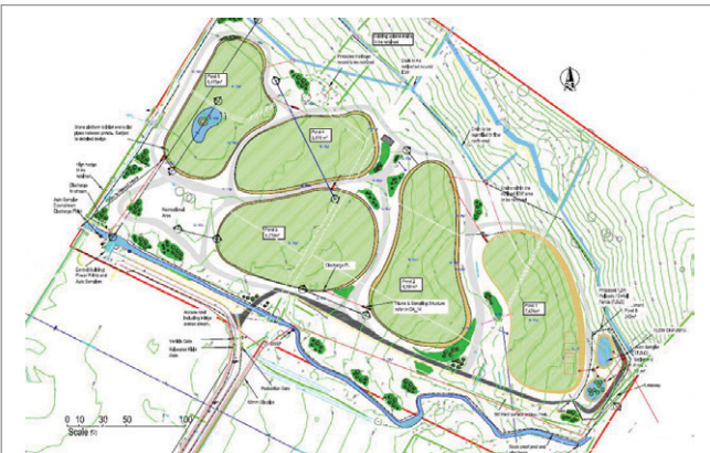
Pic 2: Site layout drawing of the wetland, which shows the layout of the various ponds - Courtesy of NI Water
