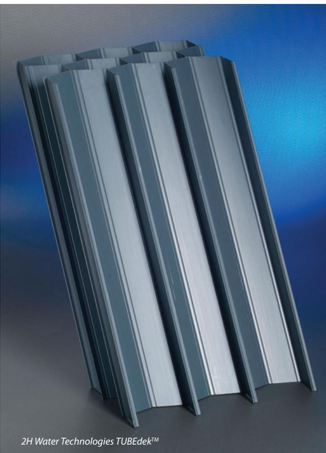
inclined angle of the tubes encourages laminar flow for efficient solids separation whilst the 'v' shape encourages a more even discharge of solids to the settlement zone below the TUBEdek™ modules.
