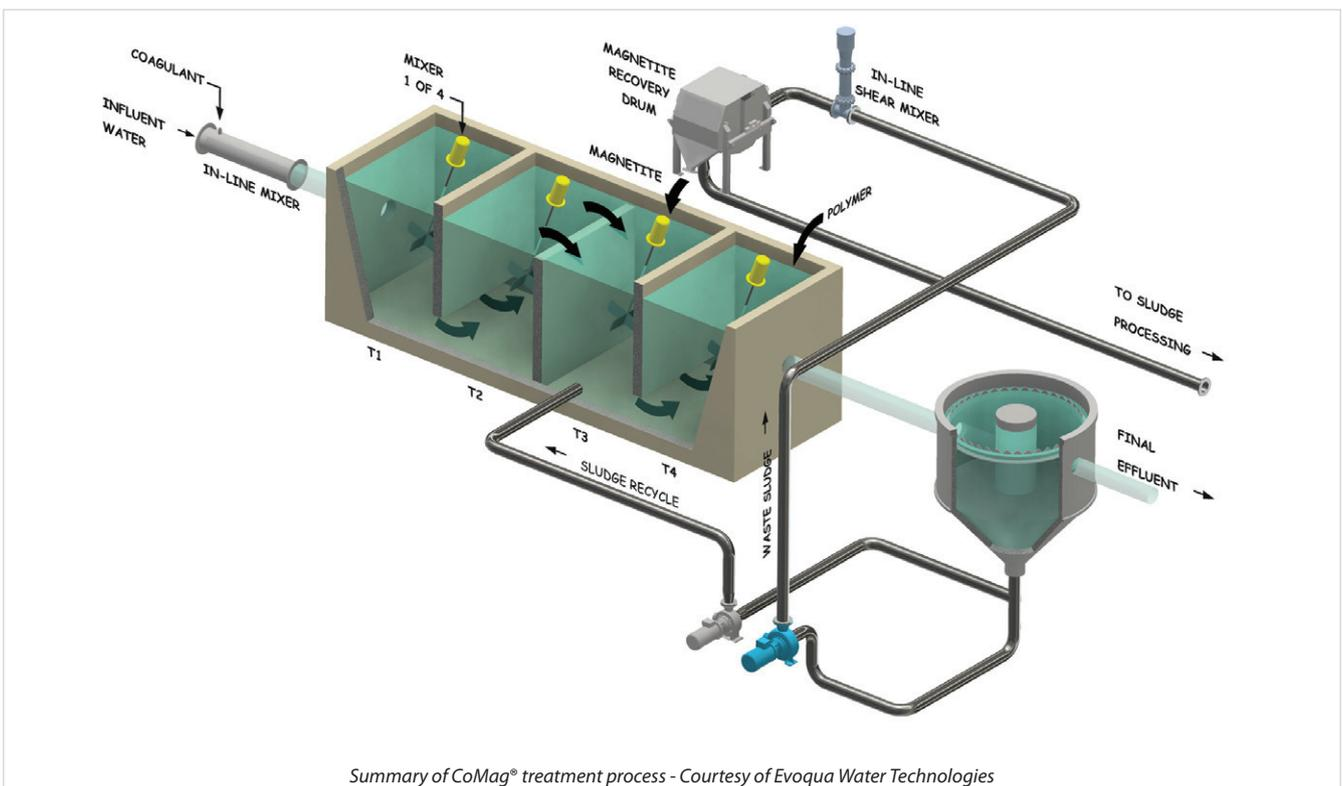
present to form insoluble ferric phosphate. The coagulant also coagulates small particles by sweep floc/charge neutralisation thus enabling the effluent total suspended solids (TSS) to be so low.
