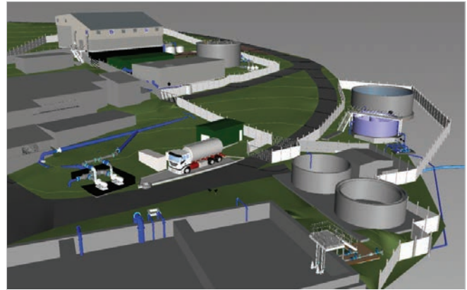
Model extract showing the existing works on the left, the new process plant on the right, and the GAC at the top of the slope - Courtesy of Galliford Try
