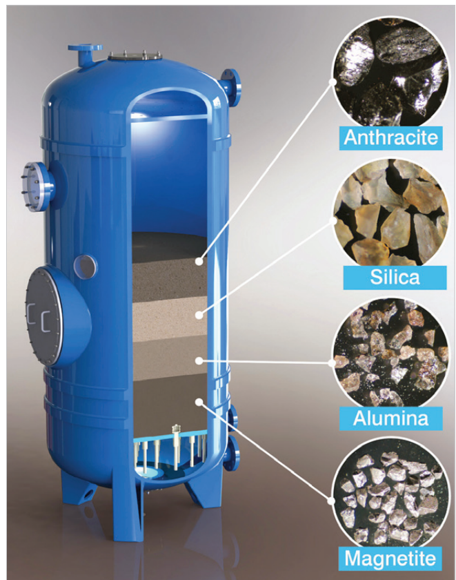
FilterClear - Four-media depth filtration (anthracite, silica, alumina and magnetite) - Courtesy of Bluewater Bio
