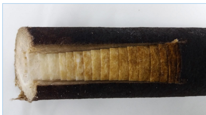
A section through the test filter shows the discolouration disappearing as the water flows from outside to in.
