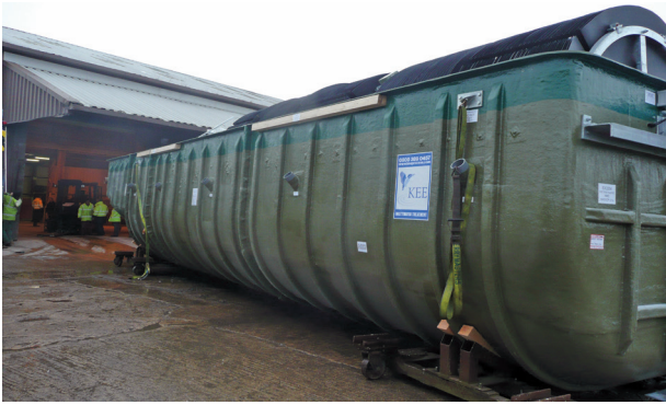
KEE NuDisc® 5000 – All factory built - 'Plug and Play' scenario.
